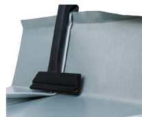
Setting up with rounded pinch pliers
