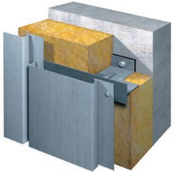
*Double or two-part substructure*
