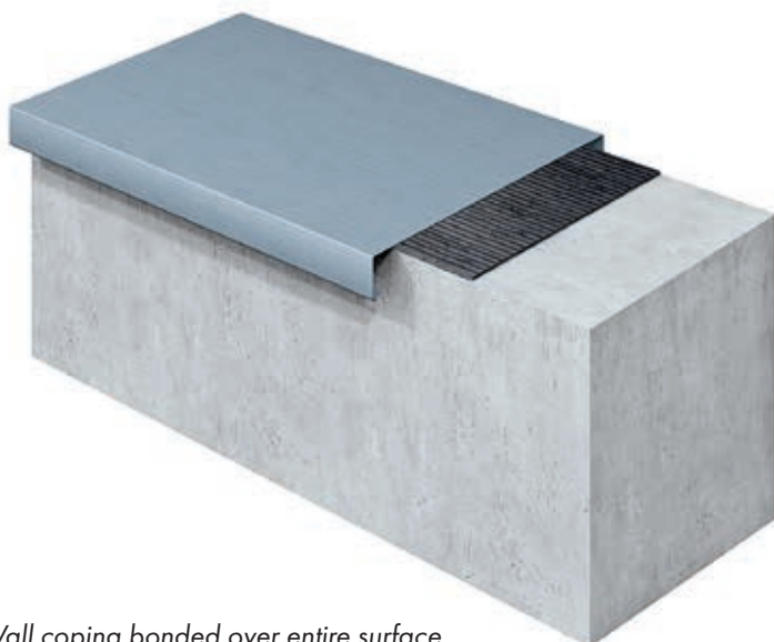
Fig. 5: Wall coping bonded over entire surface
